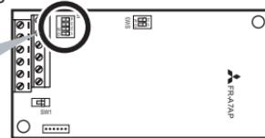
Internal terminating resistor-OFF
